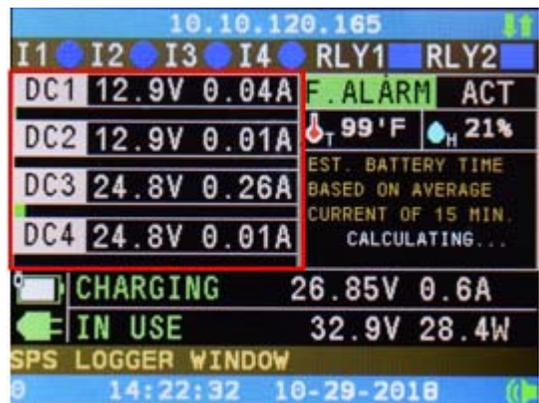
Figure 9. **Current Graph:** Four current graphs, one associated with each output channel. As current increases/decreases, current bar increases/decreases in length and graph's color is changed based on Alert current conditions as set by iOS/ Android/ Web.
