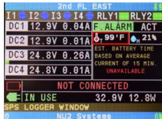
Figure 13. **Humidity:** Enclosures/closet humidity is monitored and displayed in percentage.
