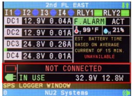
Figure 11. **Input Power Supply:** DC input voltage in Volts and total delivered power in Watts are displayed.
